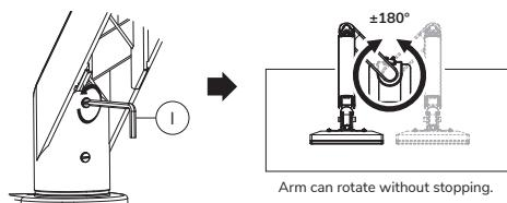
Remove or loosen the limiting screw.
