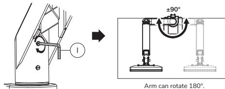
Tighten the limiting screw (do not over tighten).
