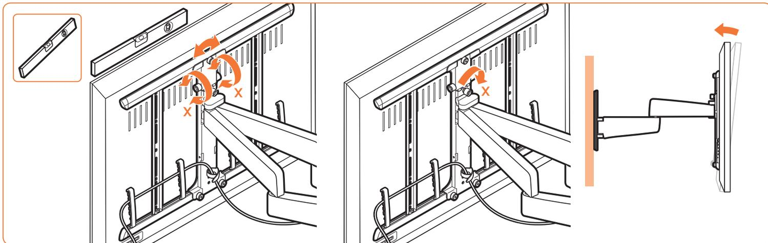
● **For tilt and level correction, turn the knobs X.**
