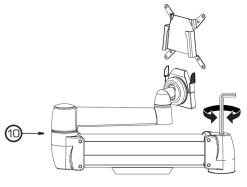
Position Arm so it is parallel to desk surface. Turn bolt clock wise for lighter monitors.
