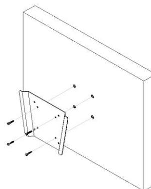
If you want to mount a screen that is VESA 75x75 mm compliant use larger of supplied screws (M4x20). Tighten the screws with the supplied Allen key.
