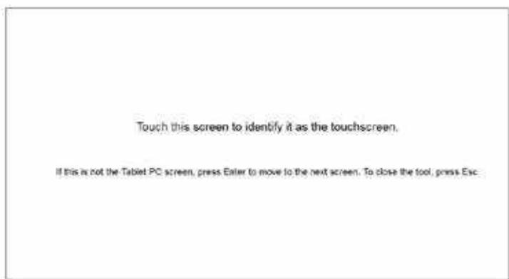
Touch the i3TOUCH and check if it recognizes touch, regardless to it's accuracy. Then check the accuracy of the touch. If not accurate, calibrate using the V-sense driver calibration. If still not accurate after calibration, go to screen resolution and choose “duplicate” again to duplicate your computer screen on the i3TOUCH.
