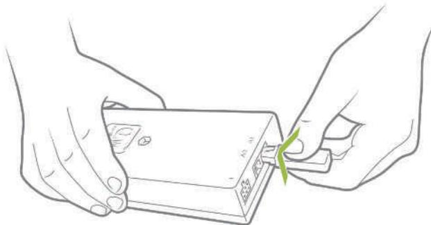
2. The Adapter is now in pairing mode. The pairing mode will last 3 minutes and is indicated by a blue flashing LED through the transparent plastic.
