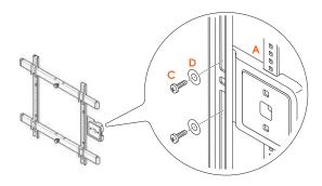
2. Screw the media box mount @ on to the TV wall mount with the bolts @ and nuts @.
