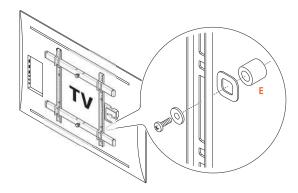
3. Attach the wall mount on the TV. Use the spacers © to create space between TV and wall mount.
