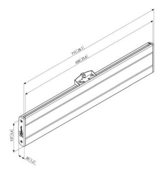
The PFB 3407 is suitable for medium- to large-sized displays up to 80 kg with a max. horizontal fitment of 650 mm. Combine this interface bar with one of the Connect-it ceiling plates (PUC 1060/ 1070/ 1080/ 1090), a Connect-it pole (PUC 2508/ 2515/ 2530) and Connect-it interface display strips (PFS 3303/ 3304/ 3305/ 3306/ 3308/ 3311) for a complete ceiling solution.
