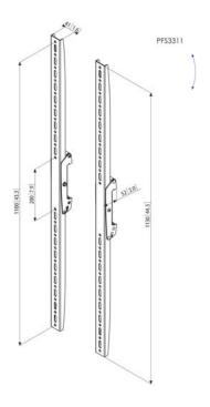
The PFS 3311 is suitable for medium- to large-sized displays up to 80 kg with a max. vertical fitment of 1100 mm. Combine these interface display strips with one of the Connect-it ceiling plates (PUC 1060/ 1070/ 1080/ 1090), a Connect-it pole (PUC 2508/ 2515/ 2530) and a Connect-it interface bar (PFB 3405/ 3407/ 3409/ 3411) for a complete ceiling solution.
