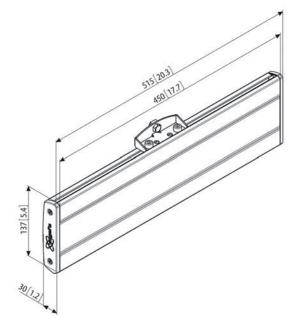
The PFB 3405 is suitable for medium- to large-sized displays up to 80 kg with a max. horizontal fitment of 450 mm. Combine this interface bar with one of the Connect-it ceiling plates (PUC 1060/ 1070/ 1080/ 1090), a Connect-it pole (PUC 2508/ 2515/ 2530) and Connect-it interface display strips (PFS 3303/ 3304/ 3305/ 3306/ 3308/ 3311) for a complete ceiling solution.
