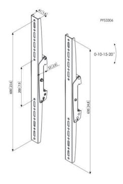
The PFS 3306 is suitable for medium- to large-sized displays up to 80 kg with a max. vertical fitment of 600 mm. Combine these interface display strips with one of the Connect-it ceiling plates (PUC 1060/ 1070/ 1080/ 1090), a Connect-it pole (PUC 2508/ 2515/ 2530) and a Connect-it interface bar (PFB 3405/ 3407/ 3409/ 3411) for a complete ceiling solution.
