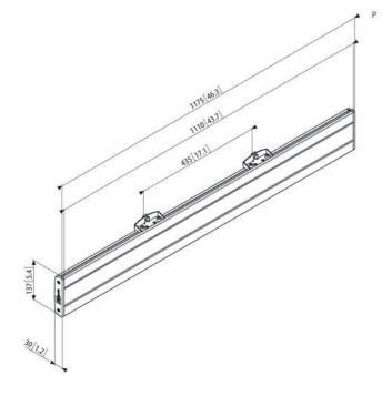
The PFB 3411 is suitable for medium- to large-sized displays up to 80 kg with a max. horizontal fitment of 1110 mm. Combine this interface bar with one of the Connect-it ceiling plates (PUC 1060/ 1070/ 1080/ 1090), a Connect-it pole (PUC 2508/ 2515/ 2530) and Connect-it interface display strips (PFS 3303/ 3304/ 3305/ 3306/ 3308/ 3311) for a complete ceiling solution.
