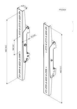
The PFS 3304 is suitable for medium- to large-sized displays up to 80 kg with a max. vertical fitment of 420 mm. Combine these interface display strips with one of the Connect-it ceiling plates (PUC 1060/ 1070/ 1080/ 1090), a Connect-it pole (PUC 2508/ 2515/ 2530) and a Connect-it interface bar (PFB 3405/ 3407/ 3409/ 3411) for a complete ceiling solution.
