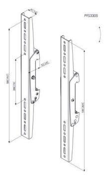
The PFS 3305 is suitable for medium- to large-sized displays up to 80 kg with a max. vertical fitment of 500 mm. Combine these interface display strips with one of the Connect-it ceiling plates (PUC 1060/ 1070/ 1080/ 1090), a Connect-it pole (PUC 2508/ 2515/ 2530) and a Connect-it interface bar (PFB 3405/ 3407/ 3409/ 3411) for a complete ceiling solution.
