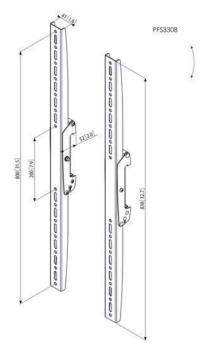
The PFS 3308 is suitable for medium- to large-sized displays up to 80 kg with a max. vertical fitment of 800 mm. Combine these interface display strips with one of the Connect-it ceiling plates (PUC 1060/ 1070/ 1080/ 1090), a Connect-it pole (PUC 2508/ 2515/ 2530) and a Connect-it interface bar (PFB 3405/ 3407/ 3409/ 3411) for a complete ceiling solution.
