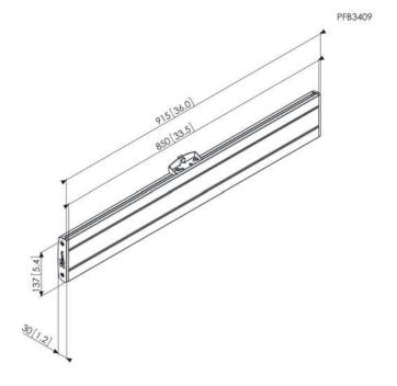
The PFB 3409 is suitable for medium- to large-sized displays up to 80 kg with a max. horizontal fitment of 850 mm. Combine this interface bar with one of the Connect-it ceiling plates (PUC 1060/ 1070/ 1080/ 1090), a Connect-it pole (PUC 2508/ 2515/ 2530) and Connect-it interface display strips (PFS 3303/ 3304/ 3305/ 3306/ 3308/ 3311) for a complete ceiling solution.
