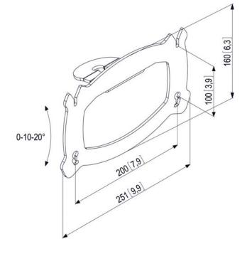
The PFI 3020 is suitable for small- to medium-sized displays (VESA 200x100 mm) up to 30 kg. This interface is equipped with a levelling and tilting function (incremental 0-10-20°). Combine this display interface with one of the Connect-it ceiling plates (PUC 1010, PUC 1030 or PUC 1040) or the truss adapter (PUC 1050) and one of the poles from the Connect-it Series (PUC 2108, PUC 2115, PUC 2308, PUC 2315 or PUC 2330) for a complete ceiling solution.
